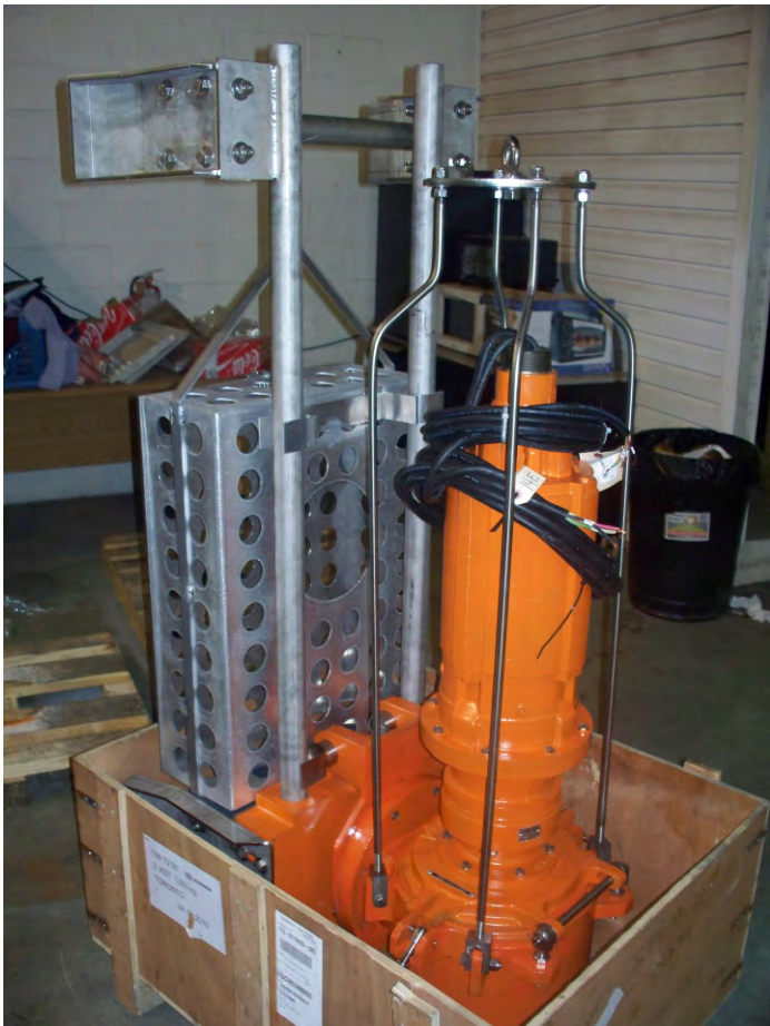
Trash Basket & Auto Coupling Slide Rails
